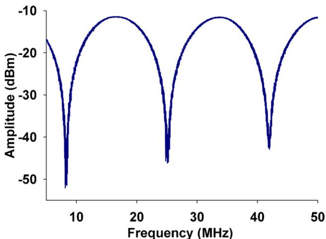
**Fig. 9.** Amplitude versus frequency plot for demineralized water obtained with the flow-through resonator at 20 °C. Resonance frequency for the first, second and third harmonics are 8.3 MHz, 25.07 MHz, 41.99 MHz, respectively.
