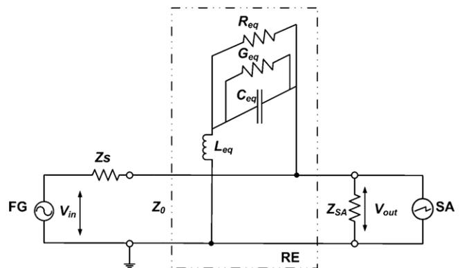
**Fig. 3.** The electrical equivalent circuit of the sensor system of Figs. 1 and 2. Parameters  $L_{eq}$ ,  $C_{eq}$ ,  $G_{eq}$  and  $R_{eq}$  represent the lumped element inductance of the resonator, the lumped element capacitance of the resonator, the conductivity of the dielectric and losses due to the skin effect in the inner and outer conductors of the coaxial resonator, respectively.
