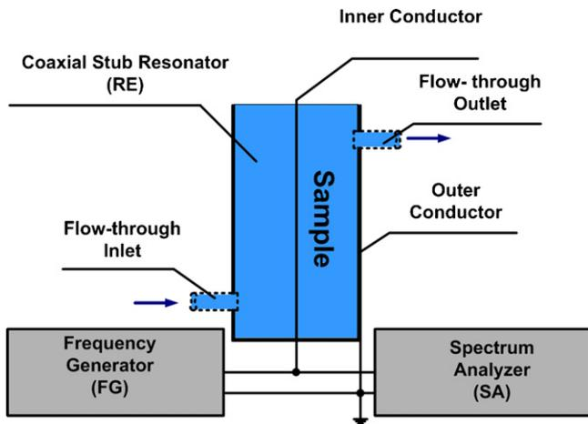
**Fig. 1.** Basic principle of the coaxial stub resonator sensing system consisting of a function generator (FG), a spectrum analyzer (SA) and the coaxial resonator (RE). The dotted structures indicate the inlet and the outlet of the flow-through resonator. Apart from lacking the in- and outlet, the design of the batch resonator is essentially the same.
