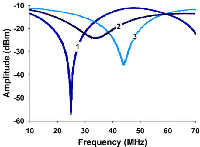
Fig. 5. Amplitude versus frequency plot for demineralized water (1), glycerol (2) and ethanol (3) as obtained with the batch resonator and the experimental set-up in Fig. 1. All experiments were executed at 20 °C.
