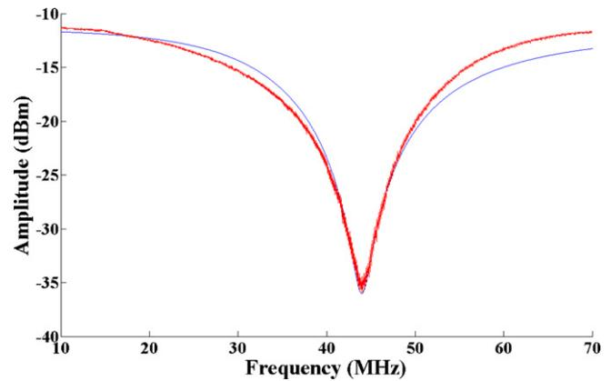
Fig. 6. Amplitude versus frequency plot for experimental data of ethanol (blue) and modeling (red) for the batch resonator using Eqs. (3)–(13) and the parameters in Table 2. (For interpretation of the references to color in this figure legend, the reader is referred to the web version of the article.)
