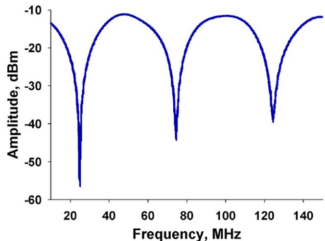
Fig. 7. Amplitude versus frequency plot for demineralized water obtained with the batch resonator at 20 °C. Resonant frequencies for the first, second and third harmonics are 24.8 MHz, 74.3 MHz and 124.7 MHz respectively.
