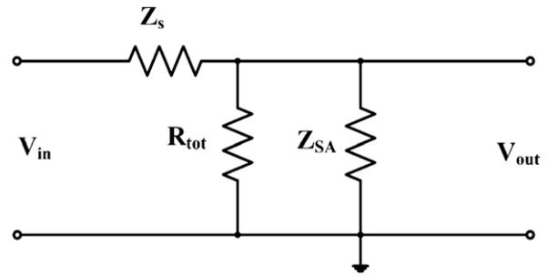
Fig. 4. Representation of the electrical equivalent circuit in Fig. 3 at resonance as a simple resistive voltage divider.
