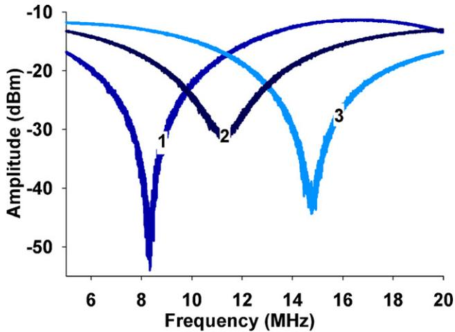
**Fig. 8.** Amplitude versus frequency plot for demineralized water (1), glycerol (2) and ethanol (3) as obtained with the flow-through resonator and the experimental set-up in Fig. 1. All experiments were executed at 20 °C.
