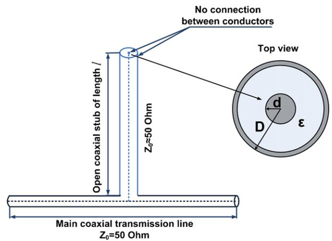
**Fig. 2.** The schematic representation of the open ended coaxial stub resonator of length  $l$  and its connection to the transmission line between function generator FG and spectrum analyzer SA.  $Z_0$  is the characteristic impedance of the transmission line and of the coaxial stub. Note that the inner and outer conductors at the end of the coaxial stub are not connected. The inset shows a top view of the coaxial stub.
